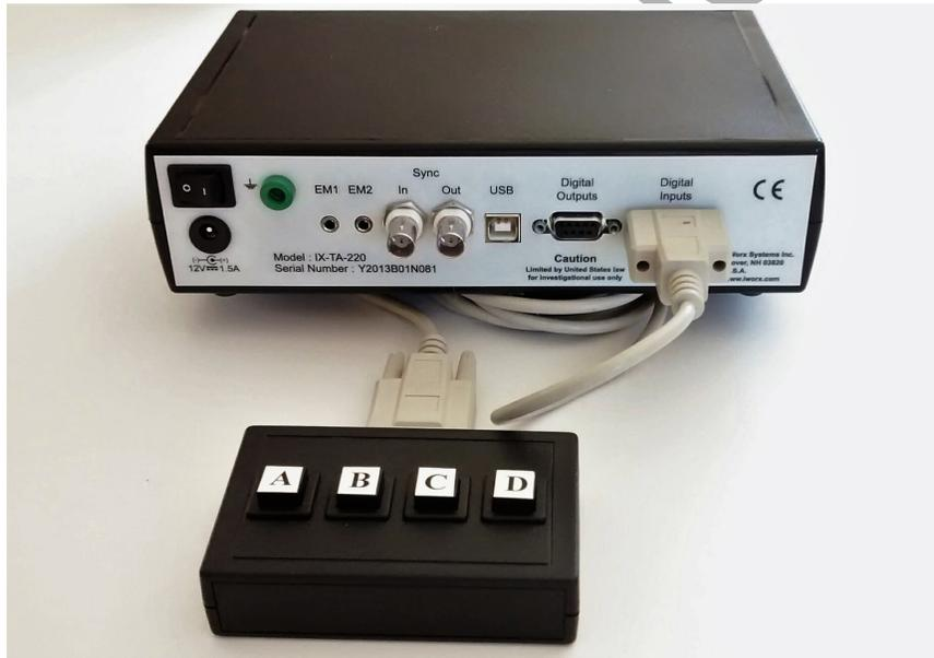
Figure HP-29-S4: The RPD 4-button response pad.
